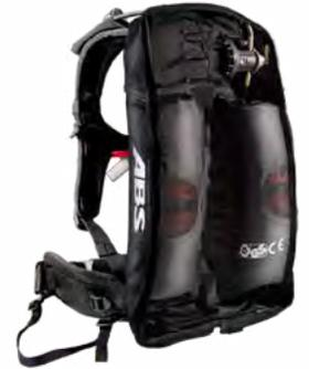
When a skier or boarder pulls the activation handle, this releases pressure that causes a pin to pierce each gas cartridge. The gas then fills the airbags, with suction and release valves taking in air from the surroundings to aid inflation.
